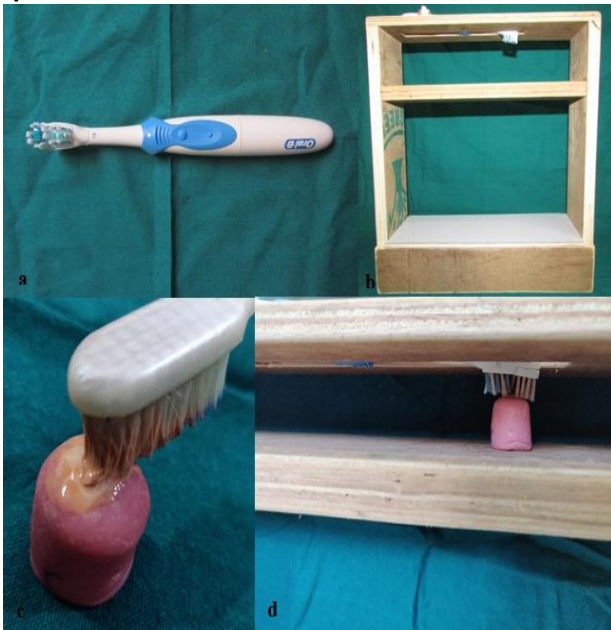
Figure 2: (A) A Powered Tooth Brush. (B) A Customized Brushing Wooden Model And A Powered Brush Attached To It. (C) Slurry Applied Over Specimen (D) Toothbrush Over Mounted Specimen.
