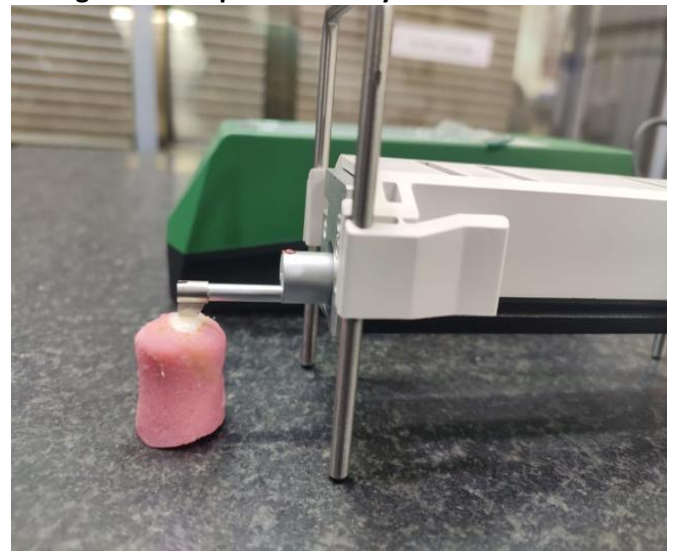
Figure 3: Samples Tested By Profilometer
