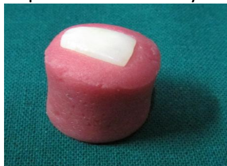
Figure 1: Specimen Embedded In Acrylic Blocks
